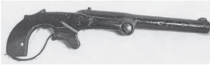
Figure 16. Right side of the “Handy Gun” showing the barrel’s tip-up lever. (Photo courtesy of Donald M. Blyth)
